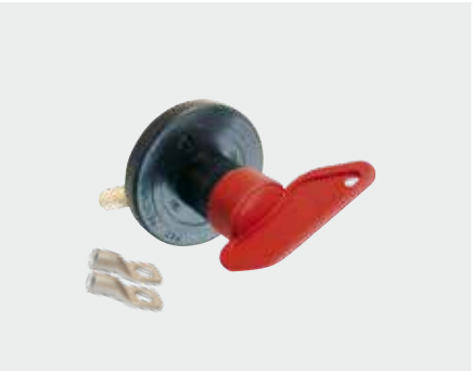
R295 223468** 003467A (without ring terminals)* Battery isolator switch 150A / 1200A (5 sec)
