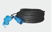
**R425/S** 212957\*\* 230V Extension cable H07RN-F, 3 x 2,5 mm<sup>2</sup> 25m, CEE plug / CEE socket + schuko socket
