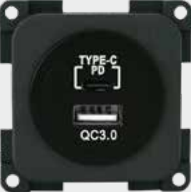
MP2USBC / ... 5V/3A USB-A + 5V/3A USB-C DOUBLE CHARGING SOCKET (INPUT 12V)
